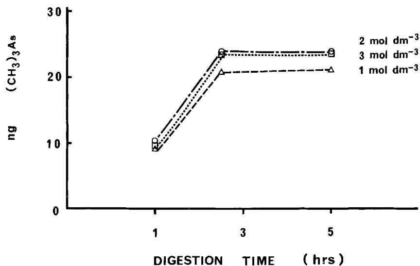
Figure 7 Time dependence of the formation of trimethylarsine through the treatment of arsenobetaine with aqueous sodium hydroxide at 85°C.
